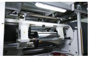
The Horizon 4.0 Triplex has been developed to laminate duplex or triplex material structures with different process technologies such as solvent- and water-based wet and dry lamination or solventless lamination. Additionally, it works as a coating machine for application of in-register solvent- and water-based varnishes and lacquers. It can also apply cold seal and pressure-sensitive adhesives.
