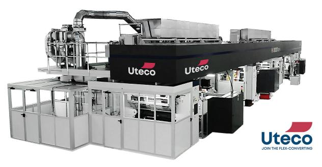
The Horizon 4.0 Triplex pays close attention to operator safety, ease of use and improved environmental performance. Operators are protected from solvent fumes due to full enclosures and the innovative ventilation system. Noise is minimised and efficiency increased thanks to the energy recovery system. Operations are also simplified via automated toolless sleeve changeovers and lifting of the coating unit trolley by automatic pistons.
